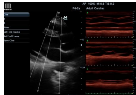
Anatomical M mode with three sample lines shows motions of three Cardiac regions simultaneously
