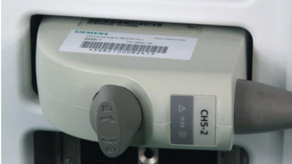
In the unlocked position, insert the transducer into the port located on the front of the system.
